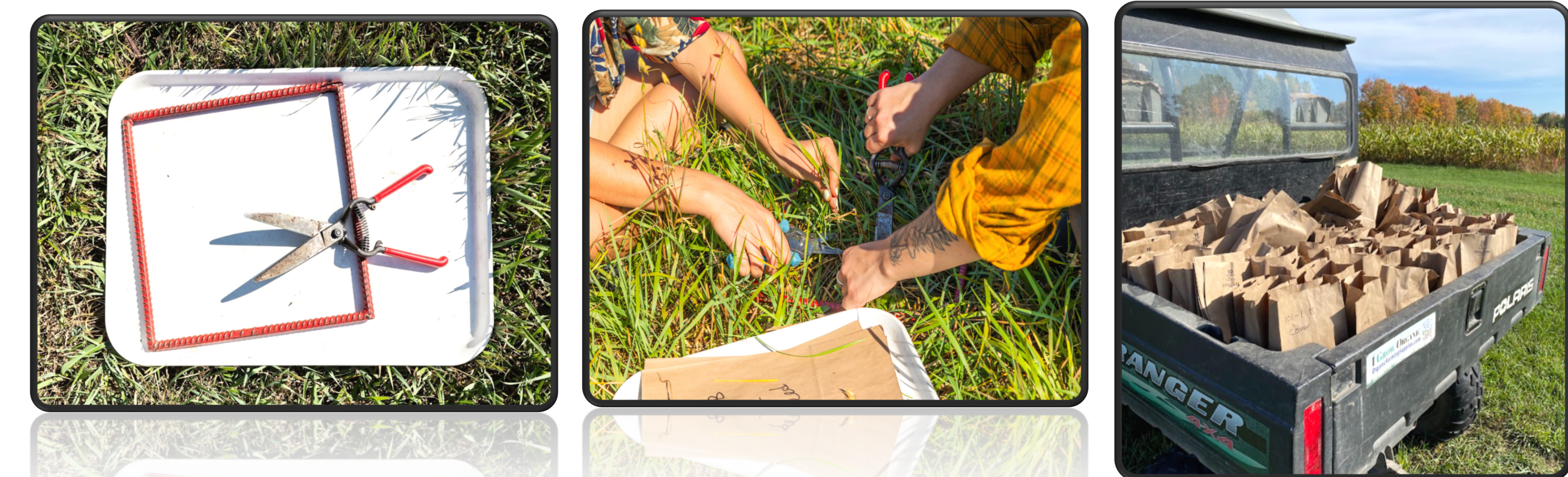
Figure 3. Methods used for biomass sampling included 1 ft 2 metal quadrants, where hand cut and sorted samples were collected in paper bags, and subsequently placed in a drying oven prior to mass determination using a digital balance.
